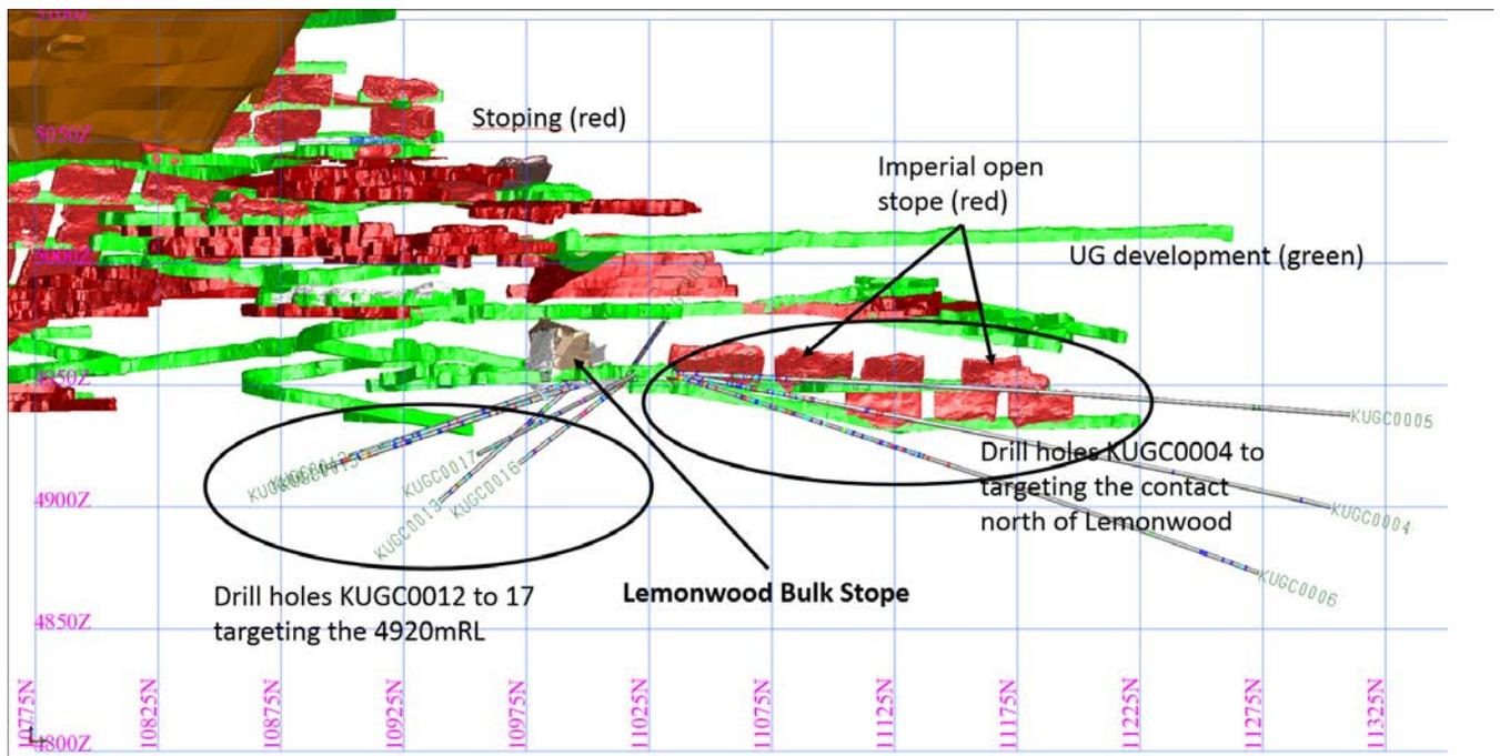
Figure 3: Long section view of the in-fill drill targeting the mineralisation in the Lemonwood bulk stope area located along the eastern contact for drill holes KUGC0001 to 6 and KUGC0012 to 17.
