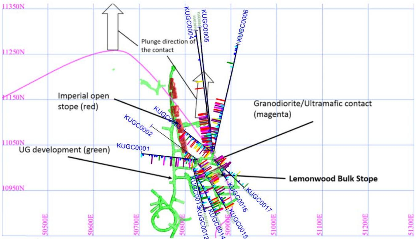
Figure 2: Plan view of the in-fill drill targeting the mineralisation in the Lemonwood bulk stope area located along the eastern contact for the drill holes KUGC0001 to 6 and KUGC0012 to 17.
