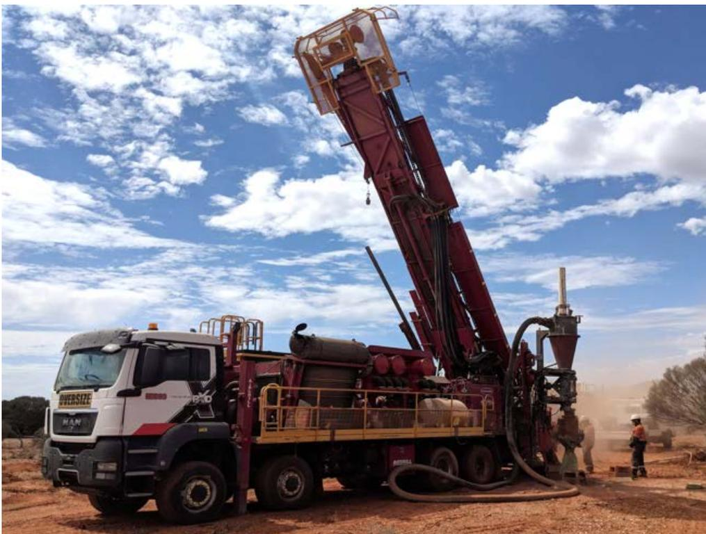
**Figure 4:** Reverse Circulation (RC) drill rig at the Centauri prospect, where drilling commenced in March 2019.
