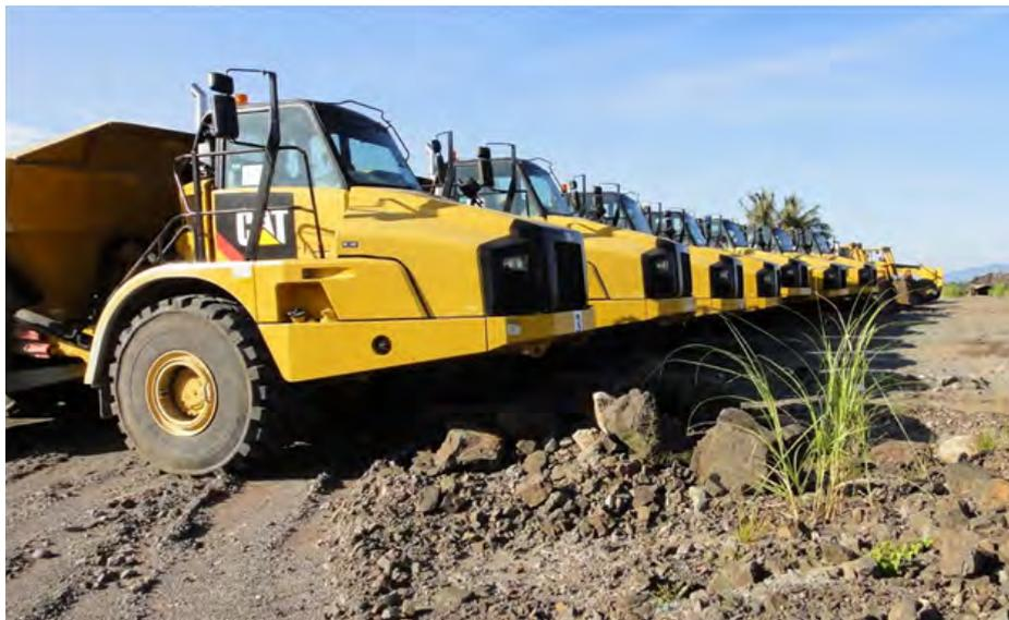
Seven 40T ADTs, one D8R dozer and a 14M grader mobilised by Galeo for mining and construction.
