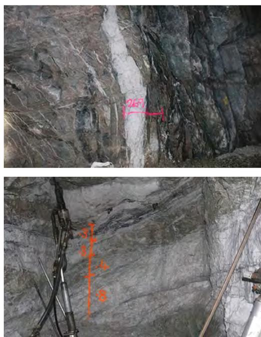
Figure 6: (Top) Aggo lode cross-cutting in the C5145 DP with values returning grades of 0.5m @ 35.7g/t Au. (Above) Kaiser – W5000 Airleg Face returning grades of 1.8m @ 21.0g/t Au.
