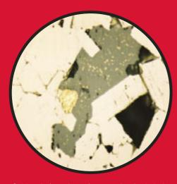
Gold grain (50 microns) on margin of sphalerite all interstitial within pyrite aggregrate.
