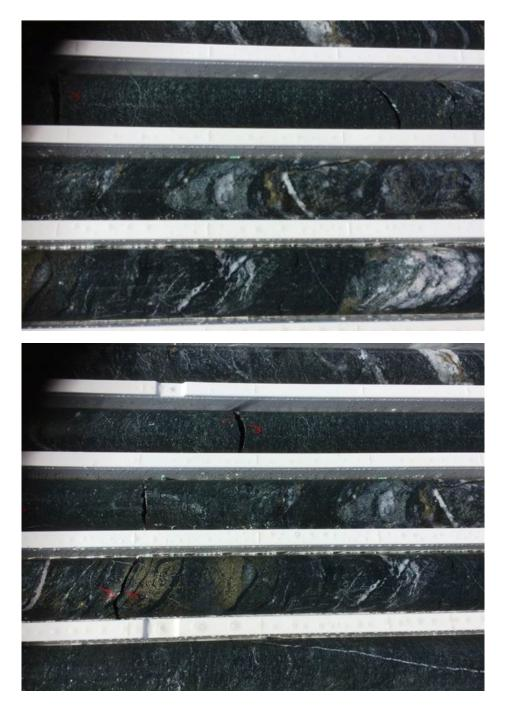
Figure 2: Drill core from SWDD0040 showing multiple, overprinting, reworked quartz-carbonate-pyrite veins hosted in magnetic dolerite (within a 4m wide zone starting at 347m). Semimassive pyrite veining present.
