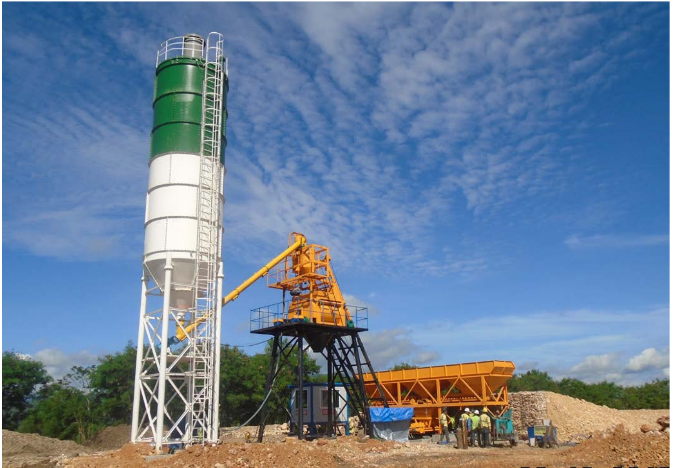
Figure 1: The concrete batch plant, constructed to support the underground mine development at Siana
