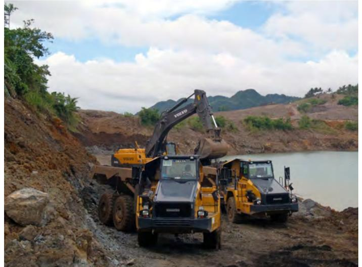
Open pit cut back – six wheel drive 40 tonne articulated trucks.
