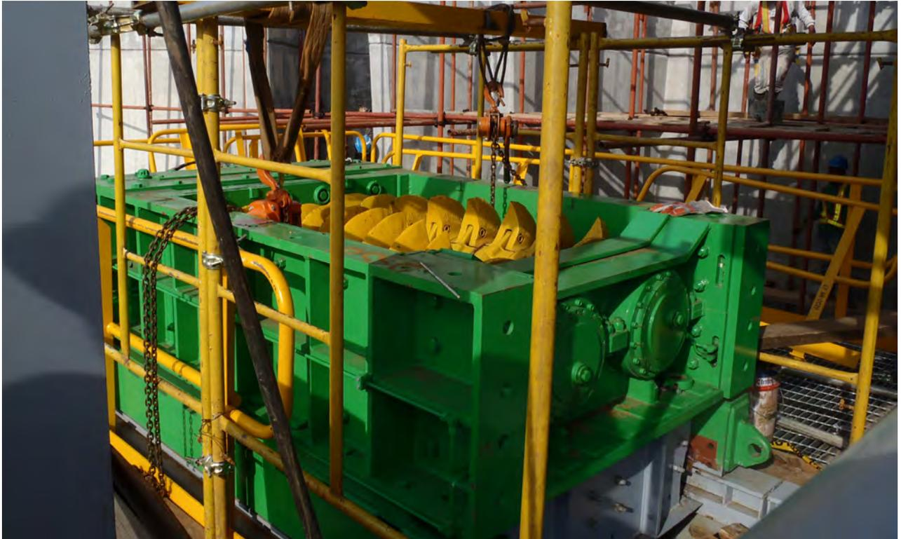
*Primary rolls crusher, specifically chosen to handle wet ore.*
