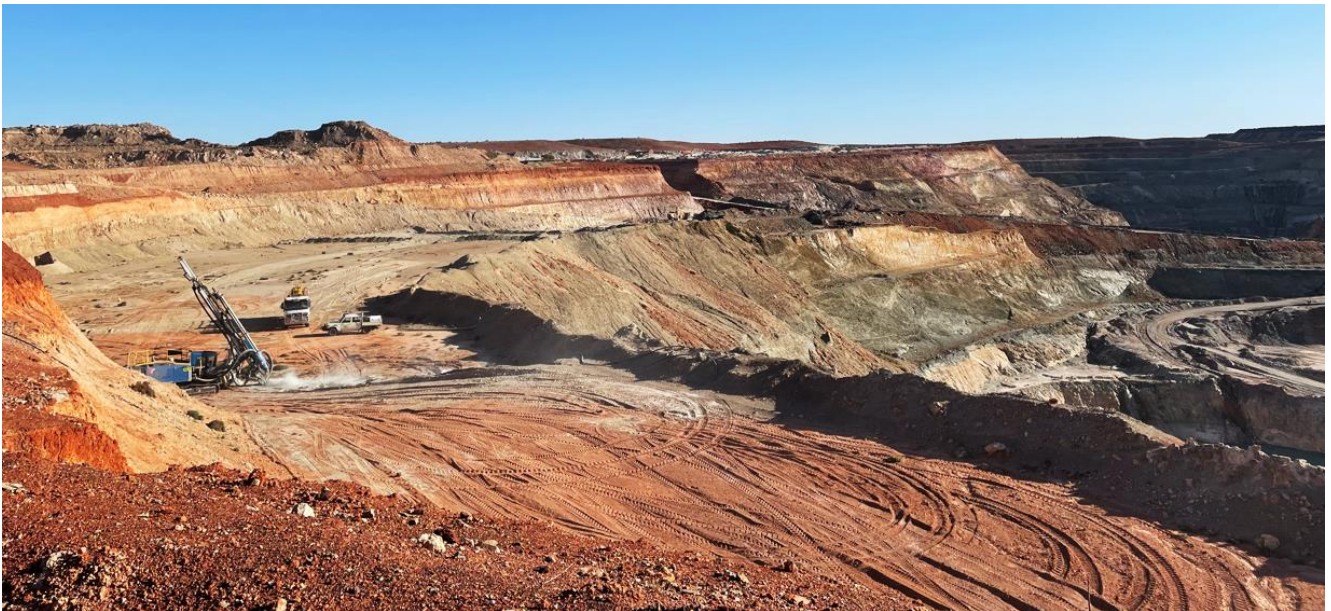
Figure 2: Mining is supported by a substantial 7m x 7m grade control program, with 62,000 metres of a 70,000-metre initial drill program already completed.
